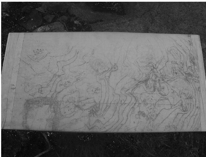
Fig 9. The map made in the field over the area according to the coordinates received from the level machine. Photographer: Alopaeus, Harry.
